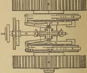
the strap the crank by its crank-pin. Though this plan of clutch may be made self-holding, it may at the same time be thrown into gear when going at great speed without the slightest shock, for the self-holding action does not come into full play till the friction-strap and its respective frictionwheel have acquired the same relative velocity.
